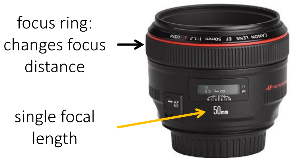
Prime lens: fixed focal length
